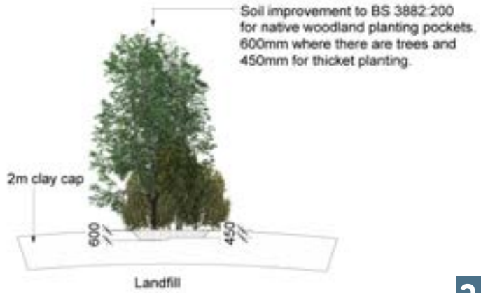
Figure 7.9 - Typical x-section of planting areas to the former landfill site
