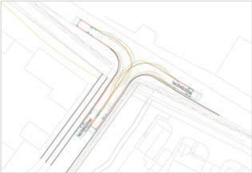
Indicative site access junction refuse vehicle swept path, refer to drawing T13522 6.2
