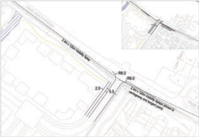
Indicative site access junction with visibility splays, refer to drawing T13522 6.1
